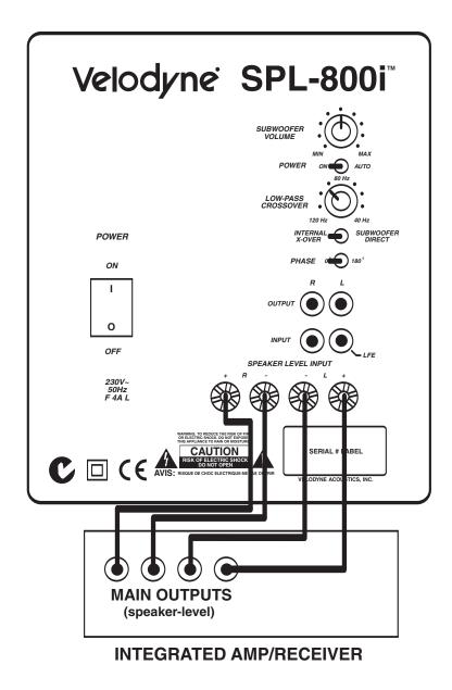
Figure 3. Installation Using Speaker-Level Inputs
